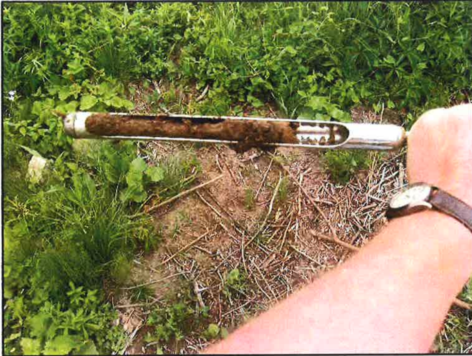
Plate 7. Soil Core from Former Greenhouse Location Showing Sandy Subsoil Terminating on Rock
