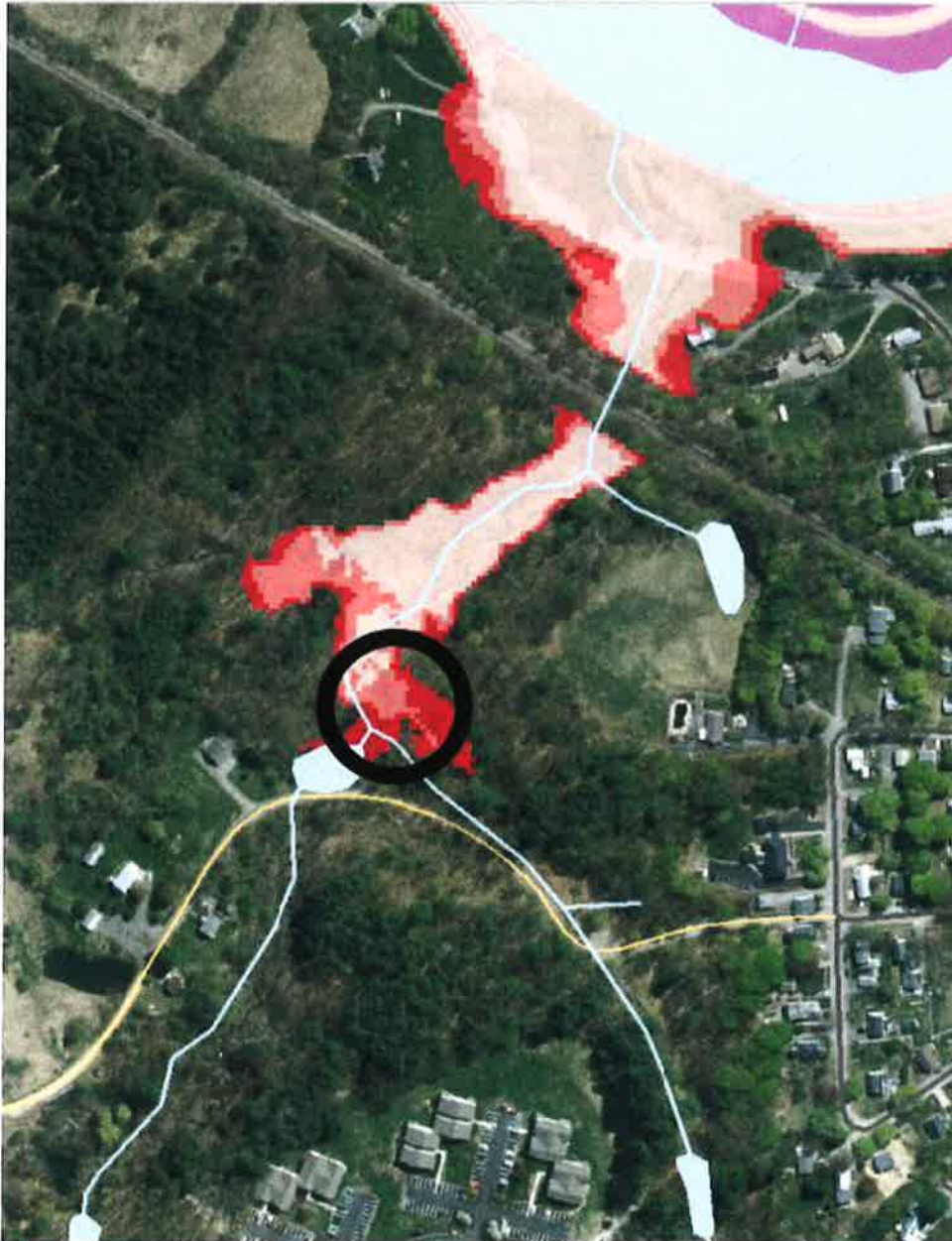
Figure 2: Sea-Level Rise + Storm Surge Map for Norris Brook Showing Location of Proposed Rose Farm Pump Station
