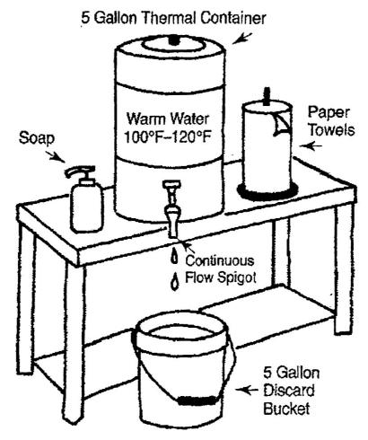
The temporary hand washing station shall consist of at least a 5-gallon insulated container with spigot that provides a continuous flow of warm (100°F- 120°F) running water, soap, paper towels, reminder sign, and a 5-gallon bucket to collect the dirty water.
