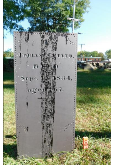
18. EWSC. F80. DT. Overview of front after scrapping with wood popsicle sticks.
