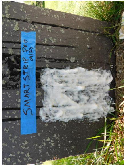
5. EWSC. F80. DT. First stripping test with Smart Strip Pro, detail.
