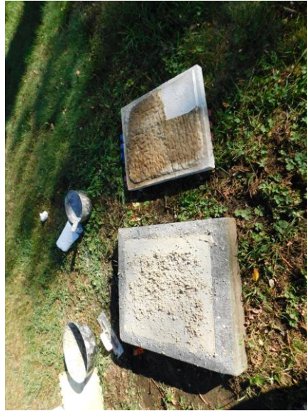
10. EWSC. A93. DT. Mortar bed on granite.
