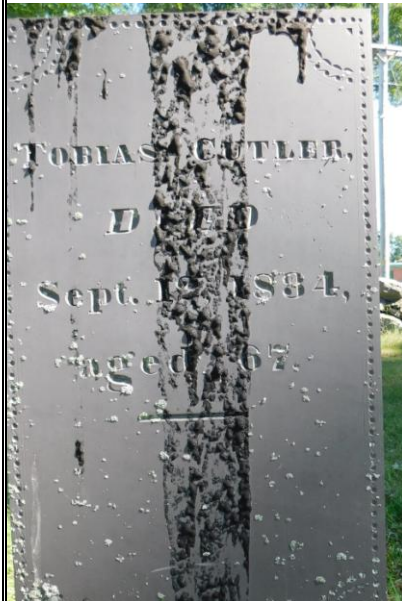
13. EWSC. F80. DT. Detail of upper front slate before scraping tar with wood popsicle stick.
