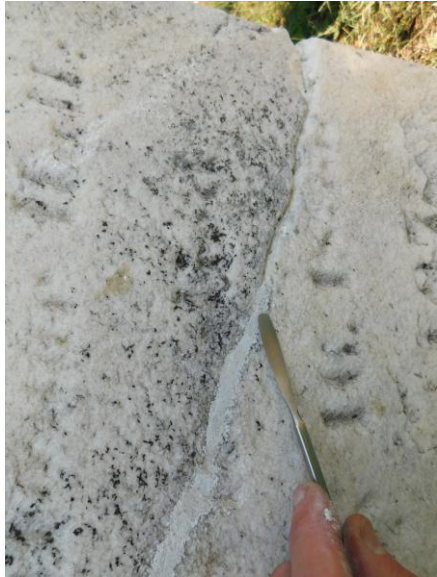
9. EWSC. A76. DT. Filling break-line with Jahn M120.
