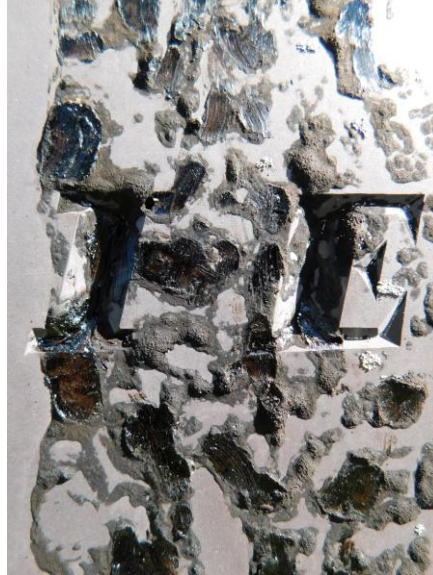
17. EWSC. F80. DT. Front detail after scrapping with wood popsicle sticks.
