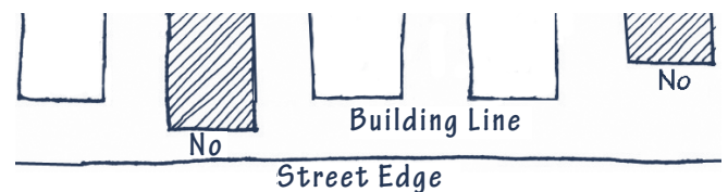
New construction should not step forward or recede back from buildings within the streetscape context.
