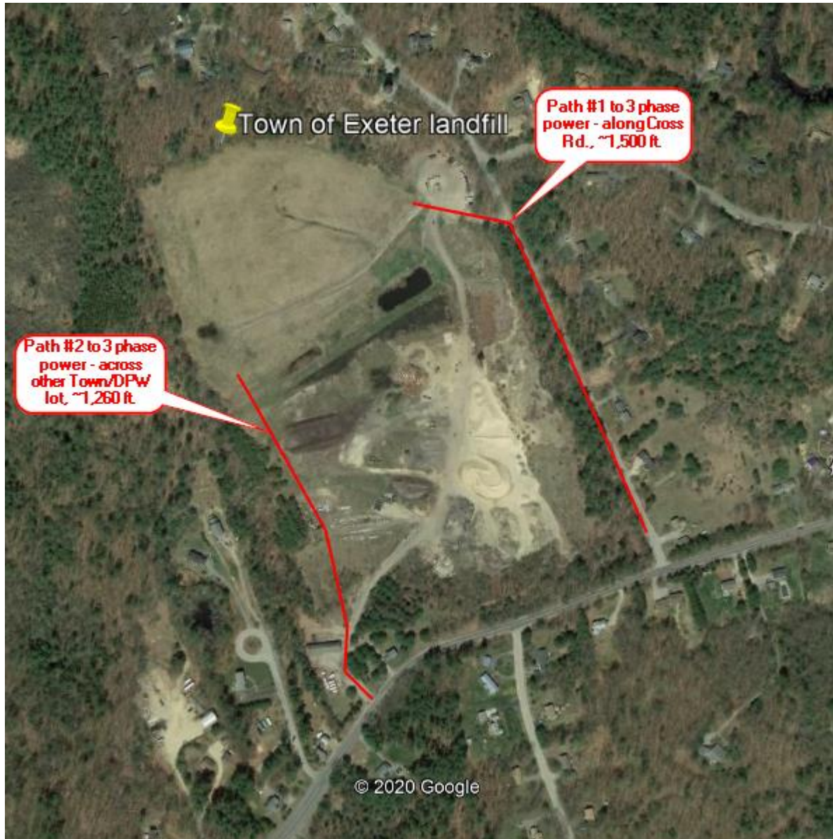
Figure 2. Potential Interconnection paths to 3-Phase Power Lines
