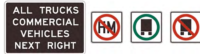
Example road signs to support/direct trucks to appropriate routes
