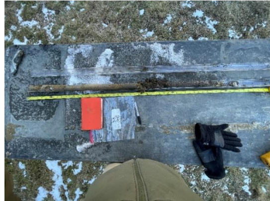
Geoprobe sample of silty sand (SM) with little gravel
