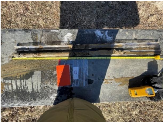
Geoprobe sample of silty sand (SM) with some gravel
