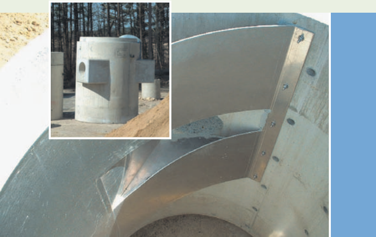
The VortSentry hydrodynamic separator is composed of a weir and baffle [above] encased in a concrete storm drain [insert]. It primarily addresses sediment, but also exhibits comparable reduction of zinc and total petroleum hydrocarbons-diesel.
