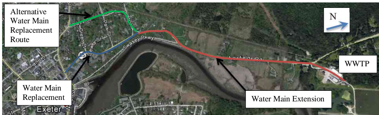
Figure 1 Water Extension Overview
