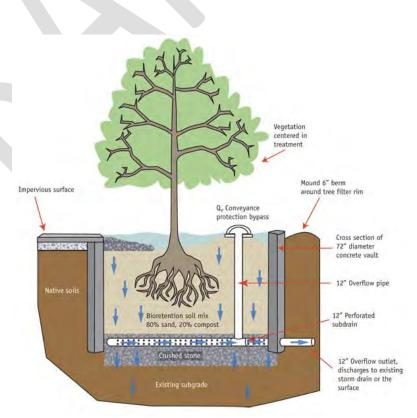
Figure 9. Tree Filter Cross-Section Detail. (Source: UNHSC, 2007)
