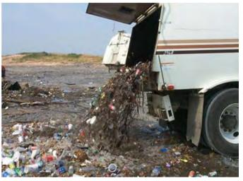
Figure 4-5. Trash from street sweeper being dumped. (Source: Chesapeake Stormwater Network)
