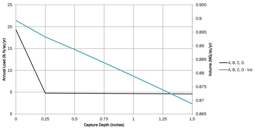
The above chart depicts the pollutant load export rates (PLERs) from the stated land use with and without the installation of the stated BMP. The PLER of the land use before treatment can be read at the capture depth of 0 inches (i.e. no BMP present). The modified PLER, after treatment from the BMP has occured, is read by reading up from the BMP's capture depth until it intersects the curve.
