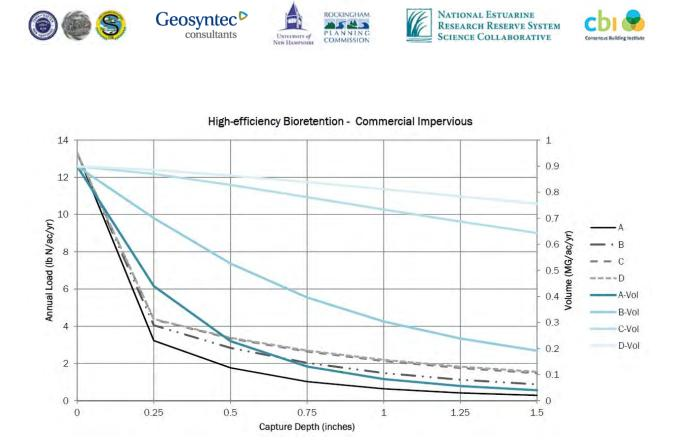
Figure 4-1. BMP Performance Curve for high-efficiency bioretention on commercial impervious areas illustrating annual exported load (lbs Nitrogen/acre/year) and volume (million gallons/acre /year) based on water quality volume (aka capture depth)
