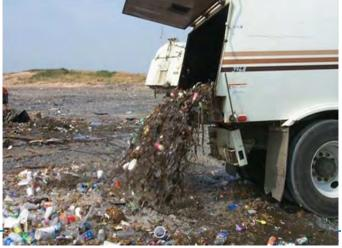
Figure 13. Trash from street sweeper being dumped. (Source: Chesapeake Stormwater Network)
