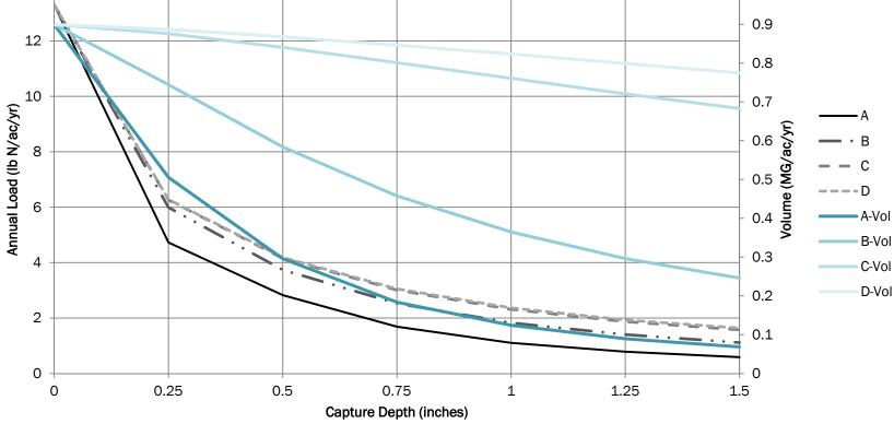
The four lines on the chart indicate the differing rates of treatment according to the soil in which the BMP is installed (hydrologic soil groups A-D). These lines will differ if the BMP includes an infiltration component, and will overlap if the BMP does not infiltrate.
