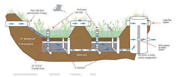
Figure 4. Gravel Wetland Cross-Section Concept Design (Credit: UNH Stormwater Center)
