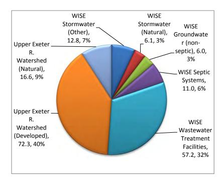
Figure 3-3. Baseline attenuated (delivered) load (tons/year) from point and non-point sources from Squamscott-Exeter watershed; Total watershed load =182 Tons per year.
