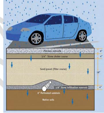
Figure 8. Porous pavement cross-section (Source: UNHSC, 2012).
