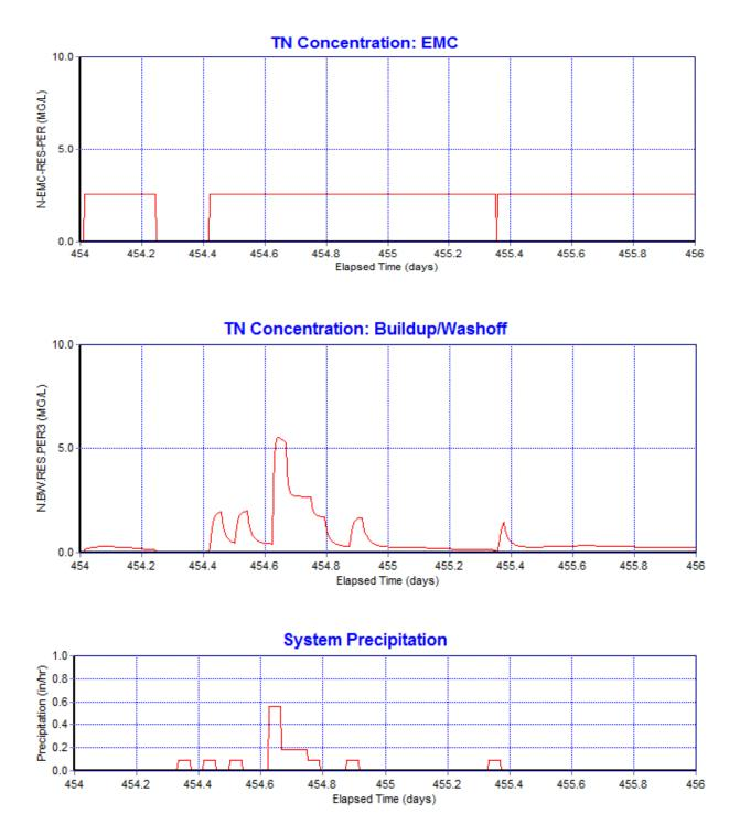
Figure 3-1. Total Nitrogen concentrations in runoff during a modeled storm event using EMC data (top) and using calibrated buildup/washoff functions (middle). Precipitation for the event is shown at bottom.
