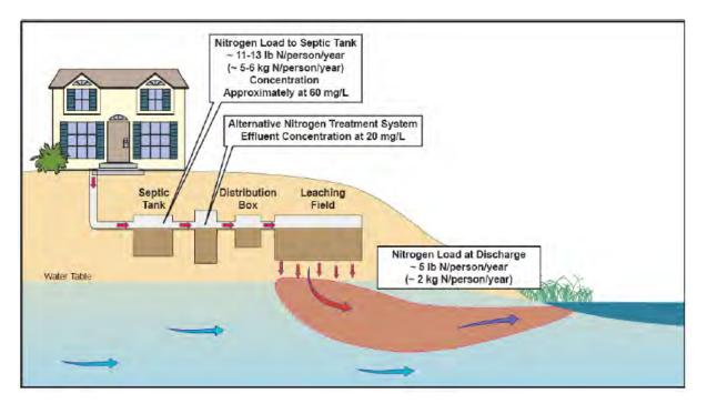
Figure 5-2. Alternative Nitrogen Septic System Upgrades
