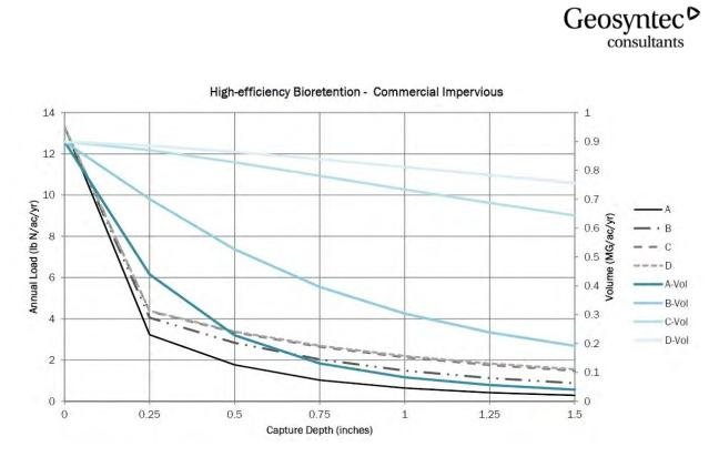
Figure 5-5. BMP Performance Curve for high-efficiency Biofiltration on commercial impervious areas illustrating annual exported load (lbs Nitrogen/acre/year) and volume (million gallons/acre /year) based on water quality volume (aka capture depth)
