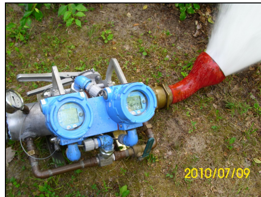
Photo of New Mag Meter at River Pumping Station and Testing the Meter in July 2010
