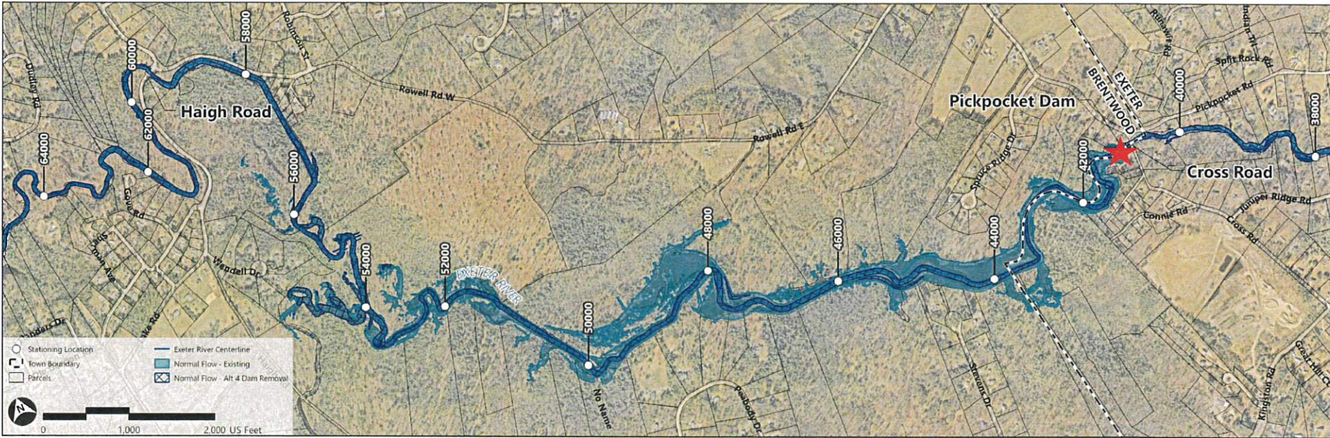
Figure 3.2-5: Alternative 4 - Dam Removal Normal Flow Water Surface Pickpocket Dam | Brentwood and Exeter, New Hampshire
