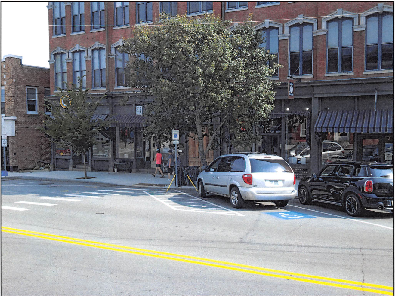
Existing designated van-accessible parking at 161 Water Street (note access aisle located on driver side).
