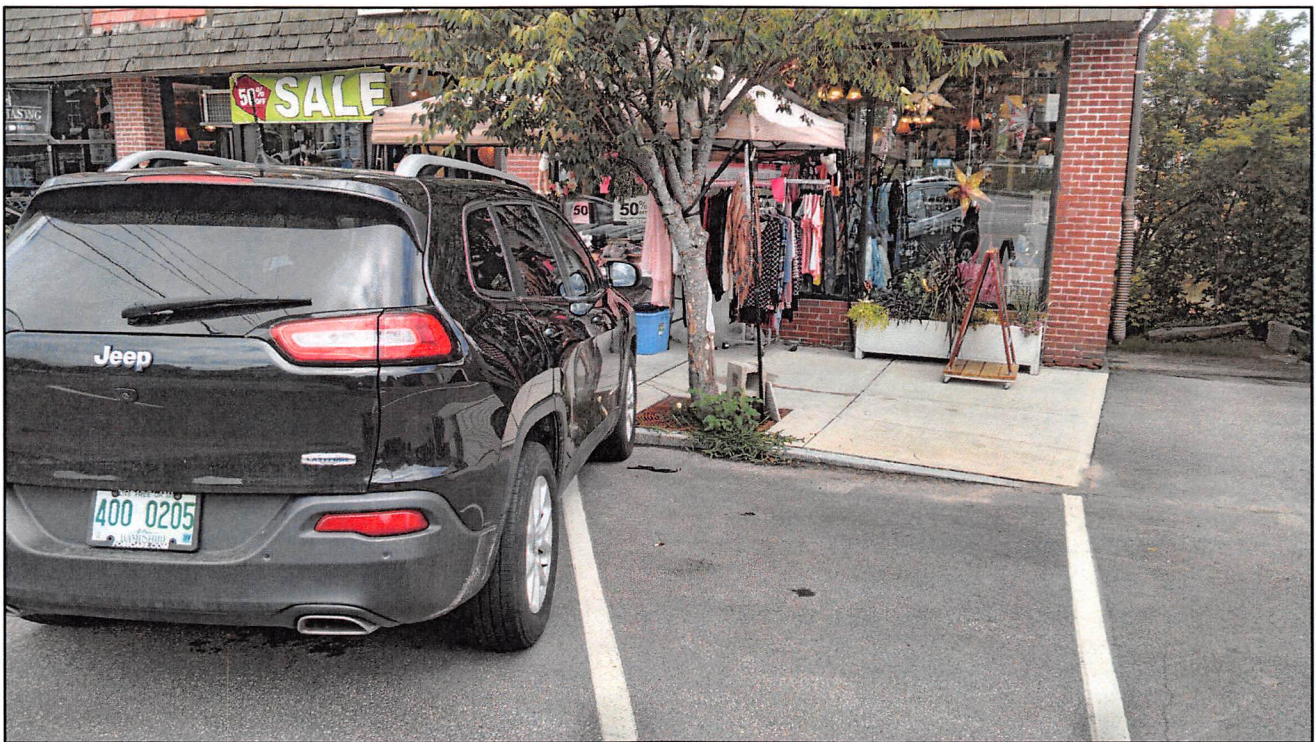
Proposed relocation (Option #1) of van-accessible parking at 85 Water Street (note access aisle would be located on passenger side of vehicle in existing gore area).
