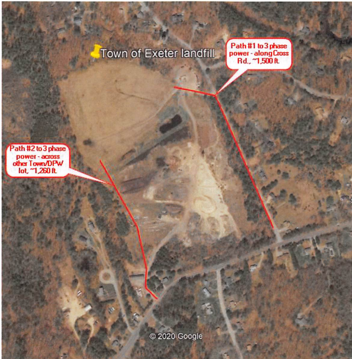
Figure 2. Potential Interconnection paths to 3-Phase Power Lines
