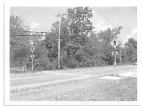
Rectangular Rapid Flashing Beacons (RRFB) were requested by residents to improve yielding compliance at the proposed Winter St crossing at Epping Rd (example shown)
