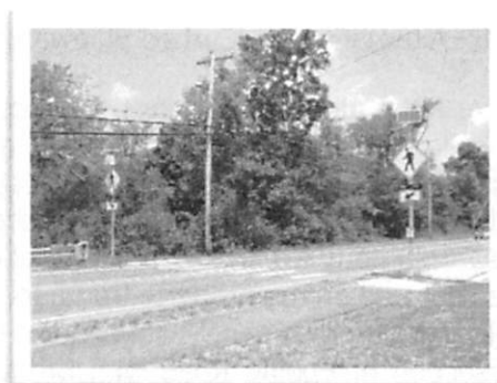
Rectangular Rapid Flashing Beacons (RRFB) were requested by residents to improve yielding compliance at the proposed Winter St crossing at Epping Rd (example shown)
