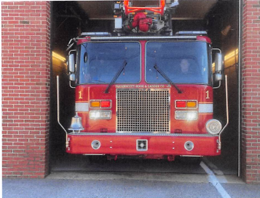
Figure 54 – Limited Clearance – this image demonstrates a lack of appropriate apparatus clearance which can complicate response and create difficult conditions to operate vehicles. This has already resulted in multiple incidents including one accident that caused $27,000 in damage and placed the aerial ladder out of service for an extended period.
