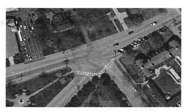
Church is located approximately 60 feet to the west of Linden Street and allows for four lanes of stacking on the church property. These conditions can cause safety concerns for motorists with numerous conflicts within a short area, confusion on which vehicle has the right of way, and limited sight lines to Front Street (NH Route 111) due to the angled alignment of the minor streets.
