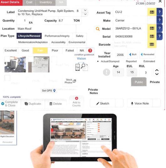
Condensing Unit/Heat Pump, Split System, 8 to 10
