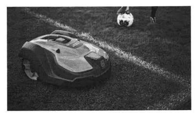
mowers have an automatic spiral-cut feature that identifies thicker patches and dedicates extra mowing time to them. This feature keeps the grass even and presentable all week. A robot mower's random mowing pattern is designed to cover the whole lawn without leaving streaks or tire marks from following a set path. There's no easier way to cut grass evenly than using a robot mower.
