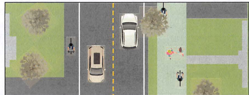
Concept B for separated bicycle facilities on Connector Streets including multi-use side path on one side of the street
