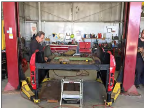
Mechanic James Pittman works on severely corroded Fire Department truck bed to return it to service.
